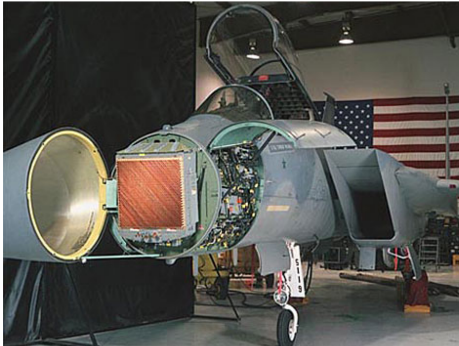
US warplanes, like this F-15C, carry active electronically scanned radar arrays in their noses that can be used as electronic warfare weapons.
