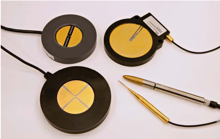
FIGURE 2.9 Examples of commercially available ultrasonic hydrophones, including membrane and probe (bottom right) designs. The overall diameters of the membrane hydrophones are about 15 cm
